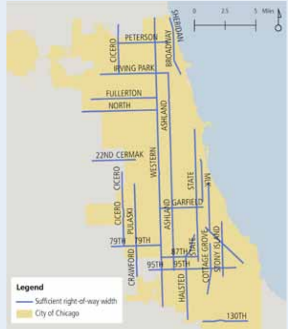
The constructability part of Phase II identified streets with consistently sufficient right-of-way width over a minimum of three miles.
