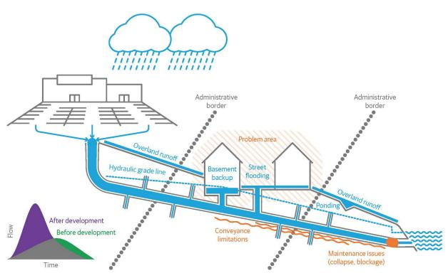
**Figure ES-1. Drainage System Schematic** Because stormwater runoff often crosses boundaries, solutions require collaboration.
